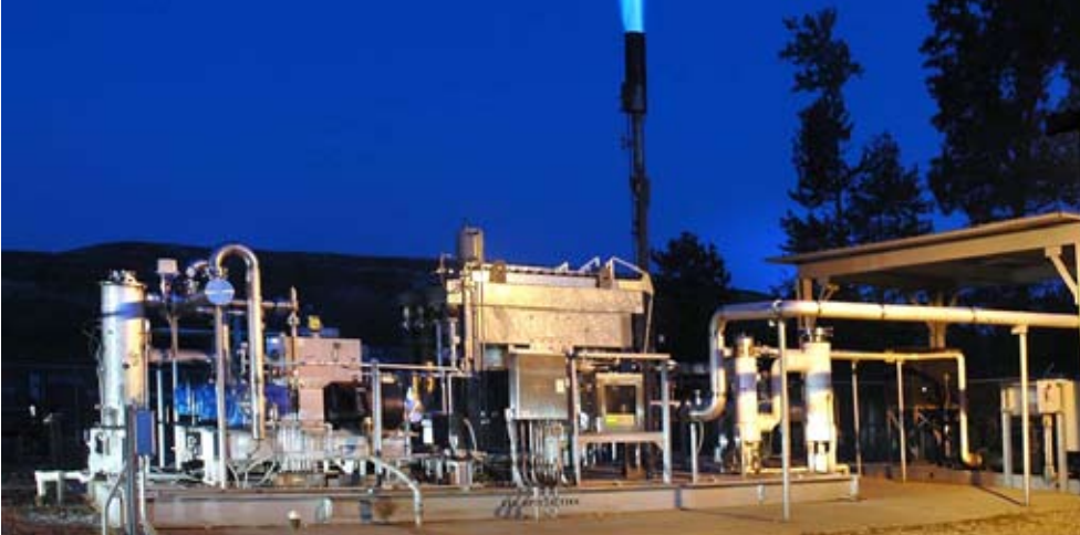
LEFT: Milliken partners with the City of LaGrange, GA to harvest methane from the landfill to replace natural gas.
